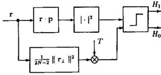
Fig. 1. Distribution-free detector for signals with unknown parameters in compound-Gaussian clutter.
