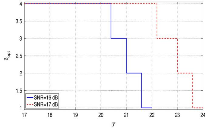
Fig. 4. Best transmit policy as a function of the estimation performance constraint with MI as the objective function.
