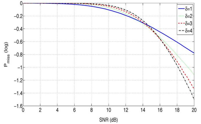
Fig. 2. Probability of target miss detection versus SNR with no constraint on the estimation performance and  $P_{fa} = 10^{-4}$ .
